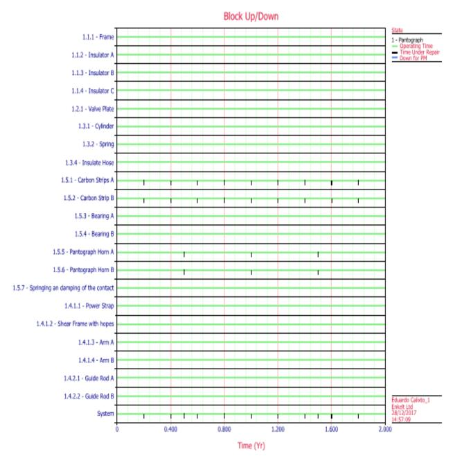
Figure 8 Pantograph Simulation result (Blocks up/down 2 years)
