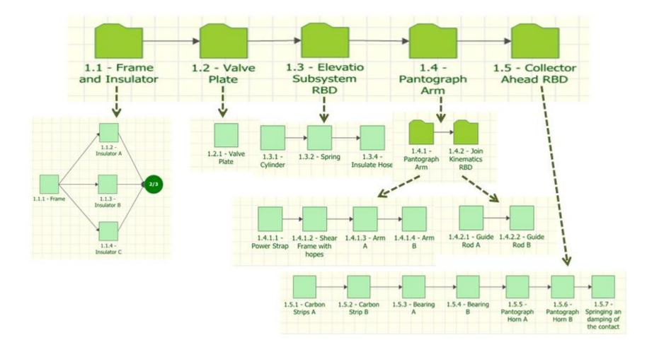
Figure 6 Pantograph RBD (Top Down configuration)
