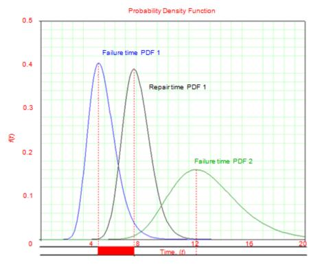
Figure 5 Monte Carlo Simulation (Block unavailability). Source: Calixto, E. et al 2015.
