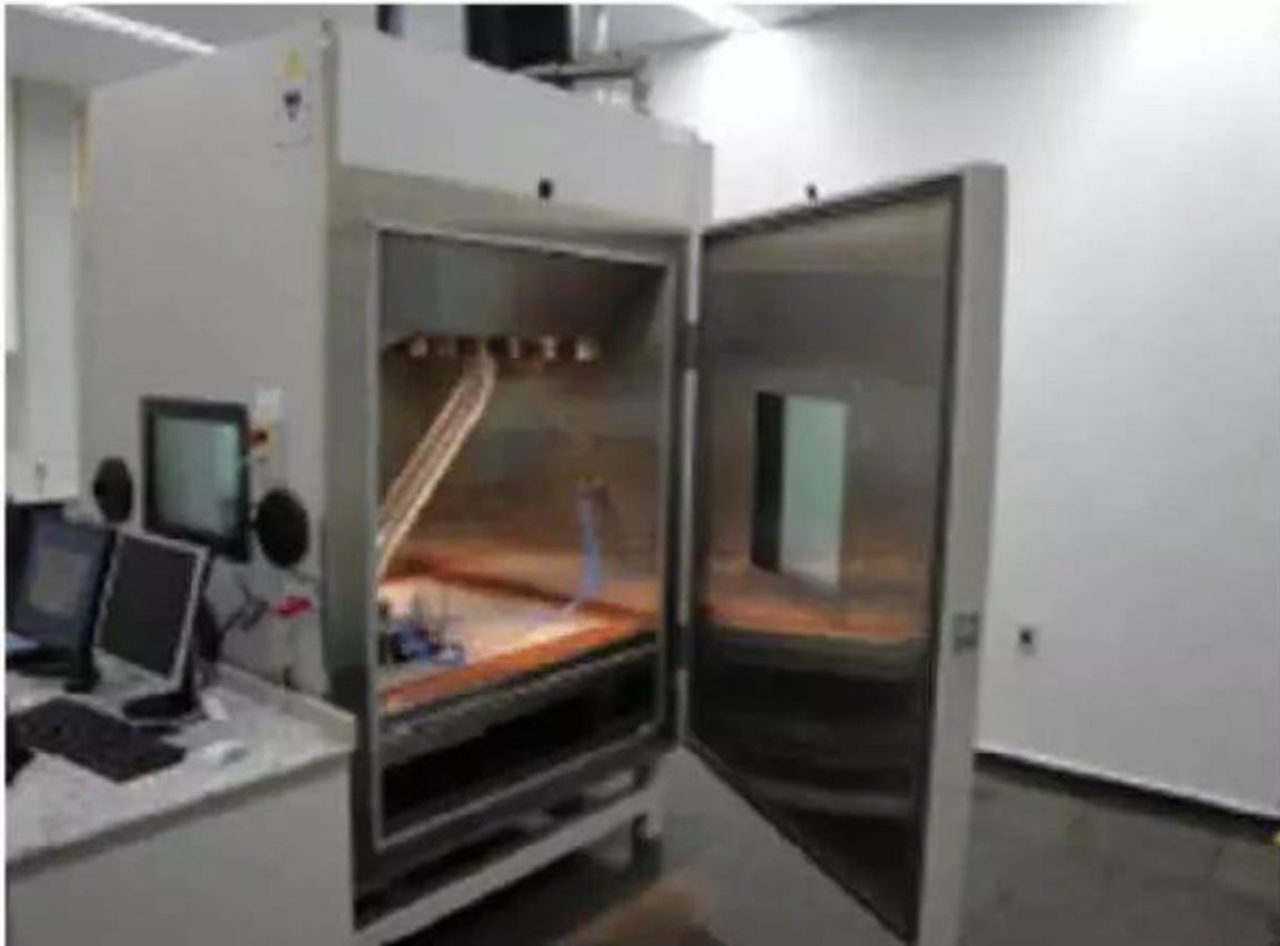
Figure 7 – ALT, HALT and HASS reliability test. Calixto Eduardo, Book RAMS and LCC Engineering for Railway Industry: Analysis, Modelling and Optimization.
