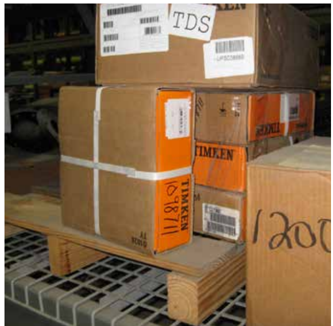
Figure 5 – Improperly stored roller bearings
