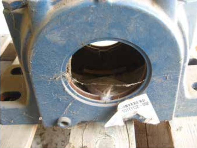
Figure 6 – Bearing housing storage open to contaminants and corrosion
