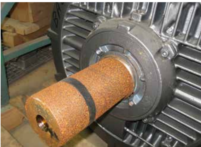
Figure 7 – Unprotected motor shaft in storage under general corrosion attack
