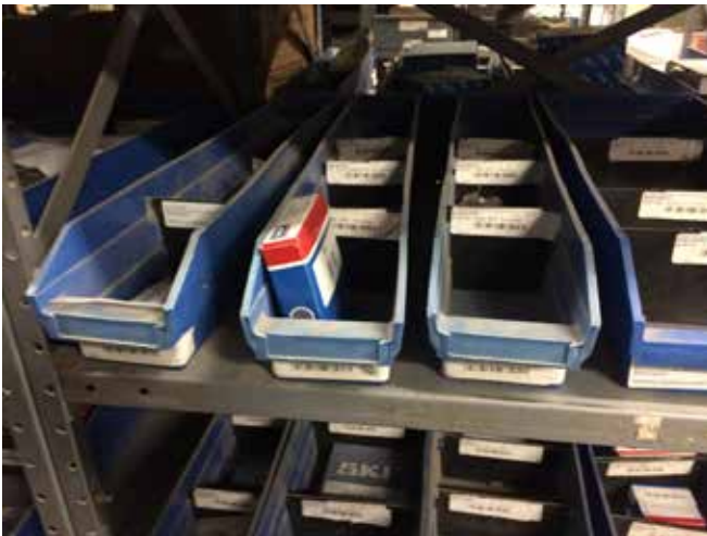
Figure 5 – Improperly stored roller bearings
