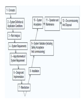
Figure 1. V diagram. Source: EN 50126.
