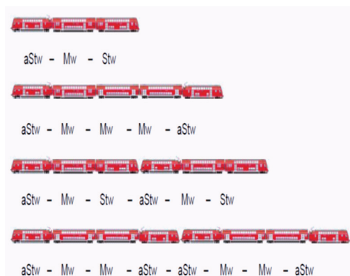
Figure 9. RAMS train configuration. (aStw = motor driver wagon, Mw = middle wagon and Stw = driver wagon).
