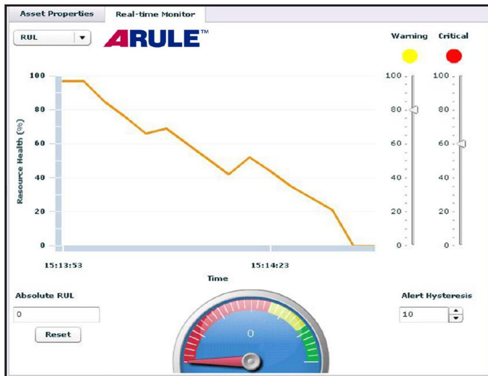
Remaining useful life representation of a system with ARULE API deployed in a Sentinel IT™ application
